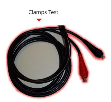
Equipment designed for the Dielectric Strength Test on electrical cables.
