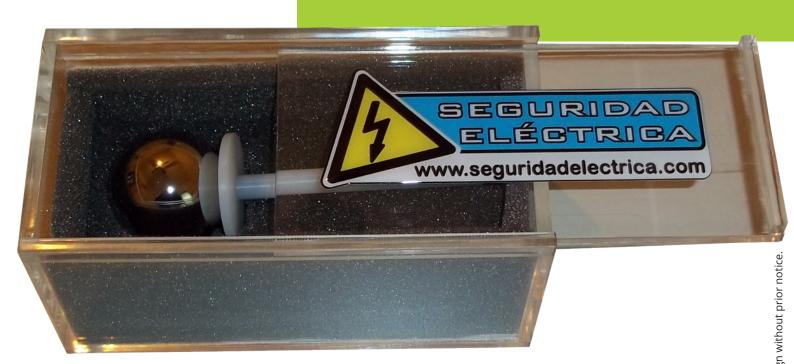
The Rigid Sphere Ø 50 mm with Guard is used to check the degree of protection provided by the wrappers mechanical equipment in compliance with the first digit No. 1 (IP1X) according to IEC 60529.
