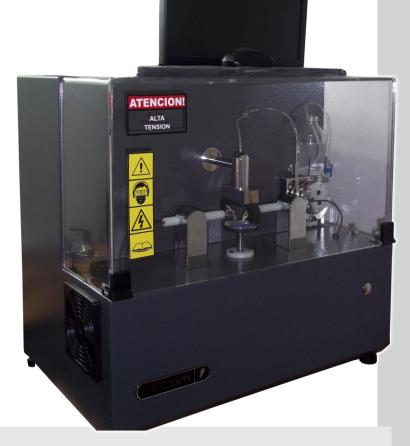
The Tracking Index Test Apparatus from Seguridad Electrica is designed to determining the Comparative tracking Index (CTI).
